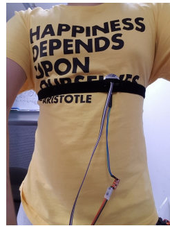
Fig. 8. The typical user scenario of our system. The left-hand figure shows the device worn on the chest. The right-hand figure shows the approximate position on the rib cage and near the diaphragm. In practical usage, the device should be worn inside the clothes to capture a high quality signal. It is reasonable because most of the chest worn wearables on the market need to contact the skin.
