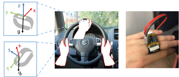
Fig. 1. The basic idea: gravitational acceleration \vec{g} in wearable coordinate frame varies when a driver hand is in different positions. When a driver’s hand is at the 12 o’clock position, the z -axis value is the major component of \vec{g} ; moving to the 9 o’clock position, the y -axis value become the major component of \vec{g}
